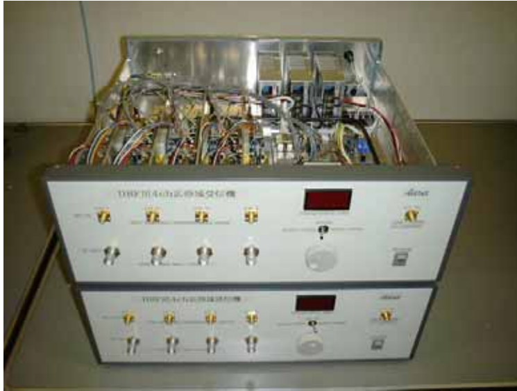
Figure 2.5: 2~8 GHz 4-channel YTF transmitter and receiver.
